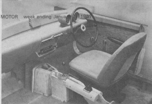
The first full-scale mock-up—in clay and wood—for the interior. Centrally placed switches, gear lever and hand brake allow for easy adaptation to right or left-hand drive.
