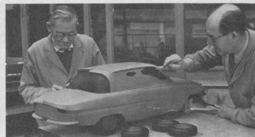
At work on a quarter-scale clay model of stage three. Alternative rear ends are being tried on the same clay model.
