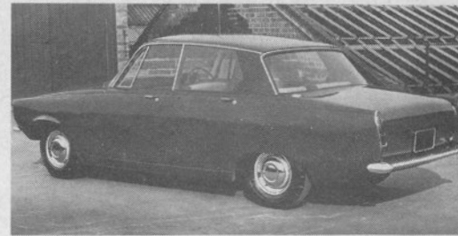
In wood at last! The first full-scale "transparent" model built of wood, and with glazed screen and windows.
